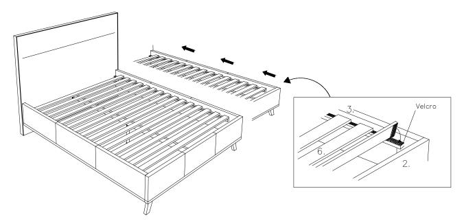
**Note**: Layout bed slats on top of Side Rail (3) start from the Footboard (2.) onward.
