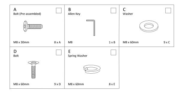
Step 1 :Attach the wood leg to the Footboard (2.) with D. M8 X 60mm, E. spring washer & G. washer then tighten before you continue to the next step.
